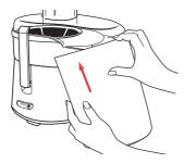
7. Take the food pusher, align the groove on the food pusher with the notch on the inside of the feed chute and slide the food pusher down into the feed chute – figure 7.
